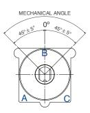
An alternative output signal to the above is an SPDT\* configuration, with "on" positions at both mechanical end stops and "off" position in the central rest position. Mechanical angle option available: ±45°
