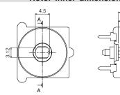
This drawing shows the rotor at 50% position, which is the standard delivery position
